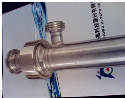
④ Installing the module head
