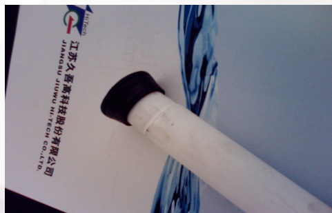
② Putting seal onto membrane element
