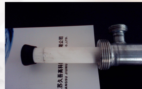
③ Putting membrane element into module
