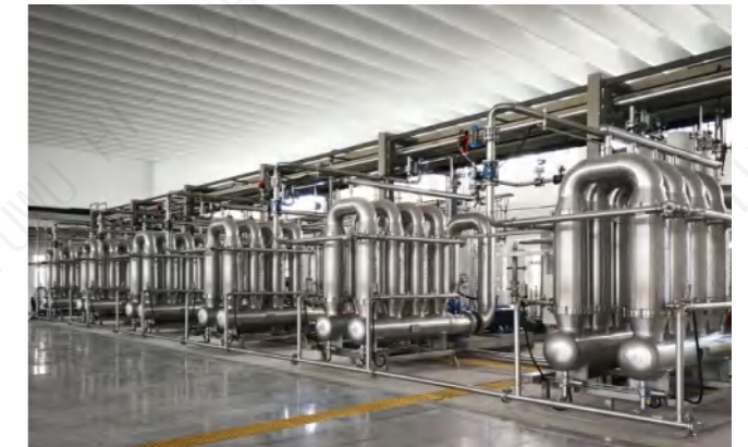
Ceramic membrane continuous filtration system of a dicarboxylic acid production enterprise in Ningxia
