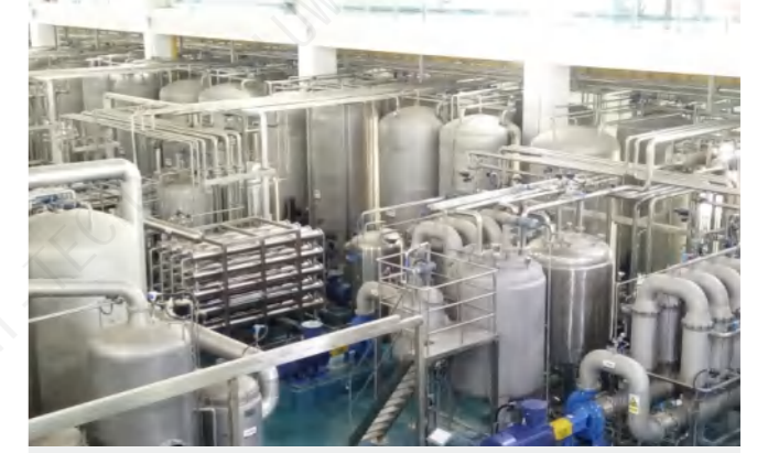
Digital extraction system of membrane method for a health wine production enterprise in Hubei province
