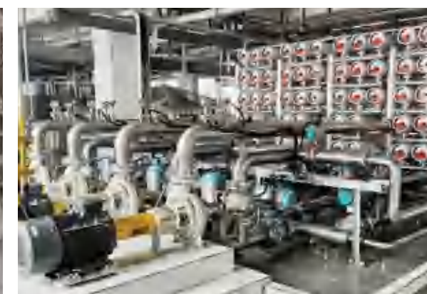
Organic membrane purification system of a vitamin producer in Hebei Province
