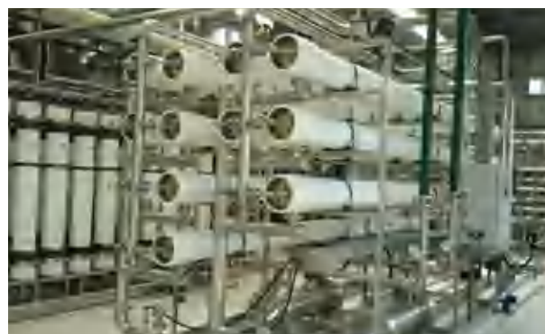
Ultrafiltration decolorization of an amino acid project in Shandong Province
