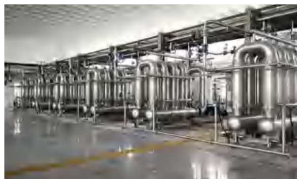
Ceramic membrane continuous filtration system of a dibasic acid producer in Ningxia
