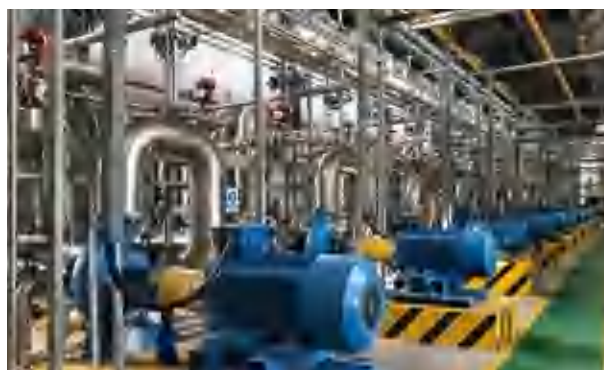
Ceramic membrane continuous filtration system of a threonine producer in Inner Mongolia
