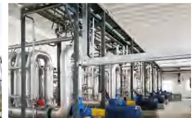
Ultrafine powder ceramic membrane continuous washing system
