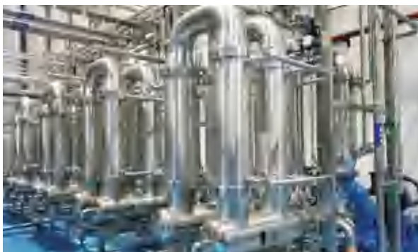
Ceramic membrane continuous filtration system of a plant extraction manufacturer in Guangxi
