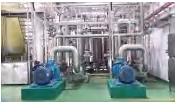
Ceramic membrane filtration system of a soy sauce manufacturer in Guangdong Province
