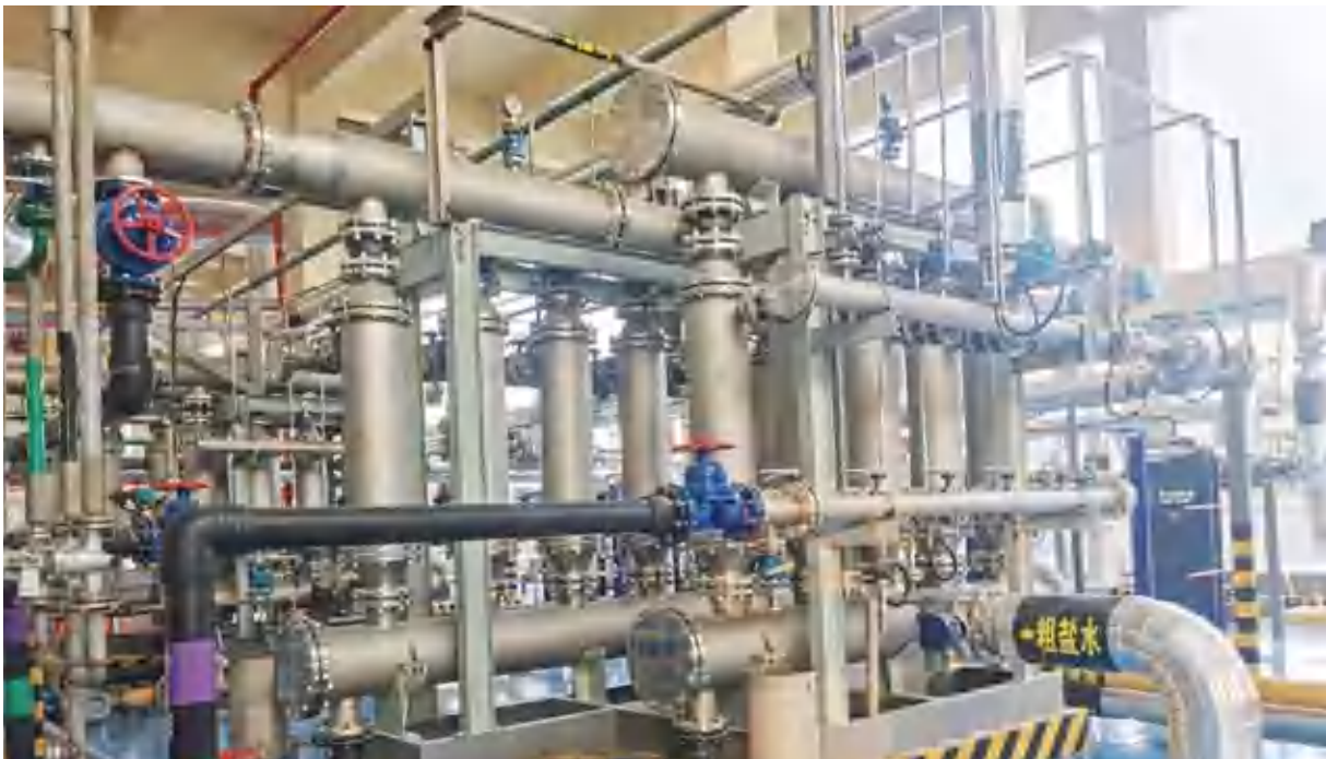
A brine refining and membrane denitrification system used by a certain enterprise in Anhui Province for an annual production of 60000 t/d tons of ionic membrane caustic soda
