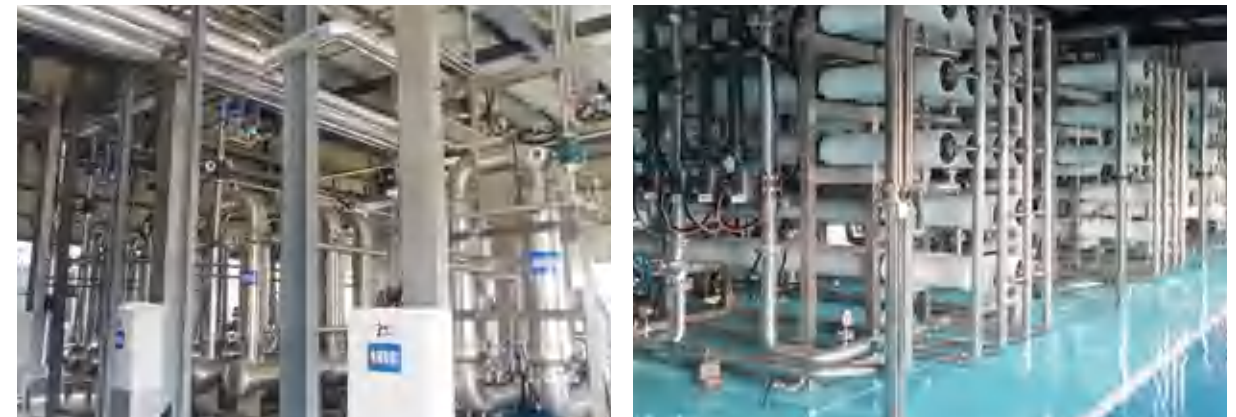
A ceramic membrane direct filtration system for 400t/d desizing wastewater from a certain enterprise in Jiangsu Province
